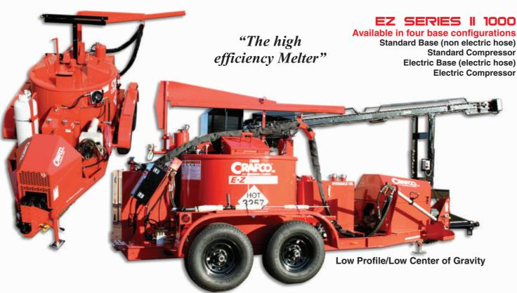
All EZ Series II 1000's come standard with a 2" sealant pump, corrosive resistant tank jacket, two part epoxy paint and one piece frame construction. Choose the unit and options that are right for you by consulting with your local Crafco representative.
